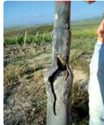
*Laborelec determined that the cable connection failure was probably due to a combination of an improper cable system design and the fact that the technology used was not the most appropriate one.*
