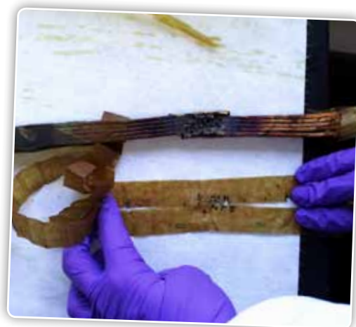
Example of an internal transformer fault (sparking) discovered through regular dissolved gasses analyses.
