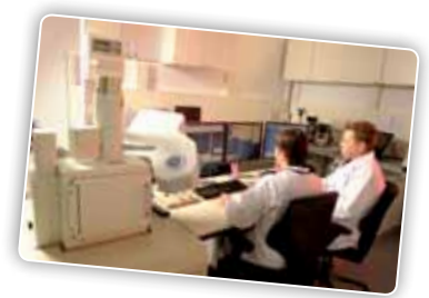
If the ICP-AES analysis indicates an increased amount of wear metals, a specific Scanning Electron Microscope/Energy Dispersive X-ray spectroscopy analysis (SEM-EDX) can be performed to determine the exact composition, quantity, shape, and origin of these contaminants.
