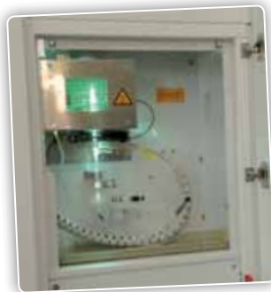
Our Inductively Coupled Plasma-Atomic Emission Spectroscopy (ICP-AES) devices enable our experts to determine the concentration of more than twenty wear or additive atoms in a lubricant or hydraulic oil.
