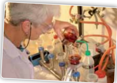
Filtering the oil in a 0.8µm filter is a routine trending analysis that helps to determine oil varnishing, external contamination, or machinery wear.
