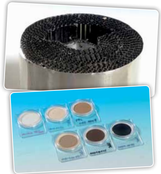
The MPC or VPI test allows to assess the risk on varnish formation in degraded oil circuit.
