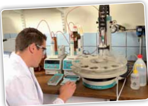
The determination of acidity is a basic analysis for trending ageing in turbine and hydraulic oils.
