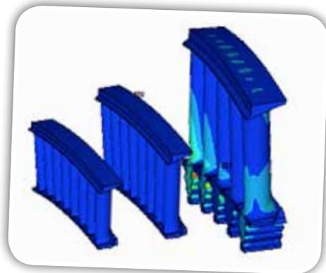
*The modification of a blade design is evaluated by calculating the distribution of resonant stress through modelling.*
