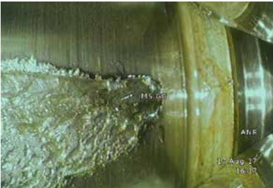
This severe bearing degradation was detected during a visual inspection. Immediate gearbox replacement was necessary due to induced degradation of neighbouring components. Such degradation, if undetected, could have led to abrupt seizure, with potential dramatic consequences including shaft rupture or gearbox total loss.
