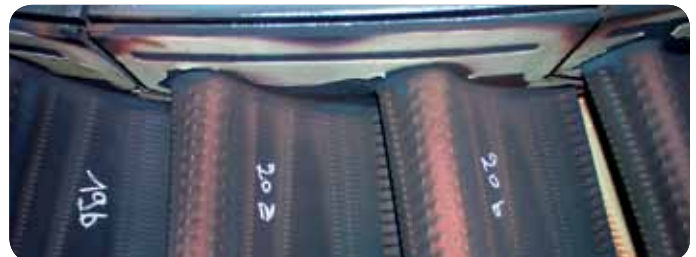
Remote monitoring identified a potentially dangerous temperature increase which led to the remedial action avoiding damage to the stator blades.
