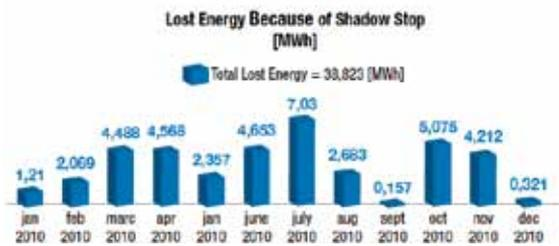
Find out how much energy is lost due to stopping a wind turbine in order to reduce stroboscopic effects.
