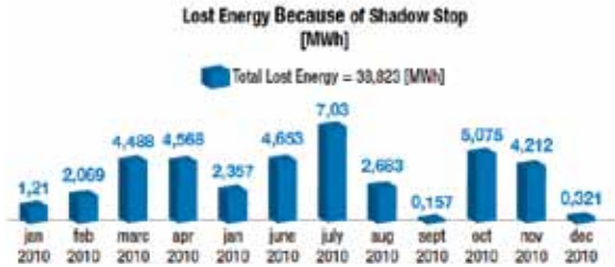
Find out how much energy is lost due to stopping a wind turbine in order to reduce stroboscopic effects.
