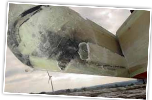
Blades and other turbine components are exposed to lightning strikes and therefore require appropriate protection.
