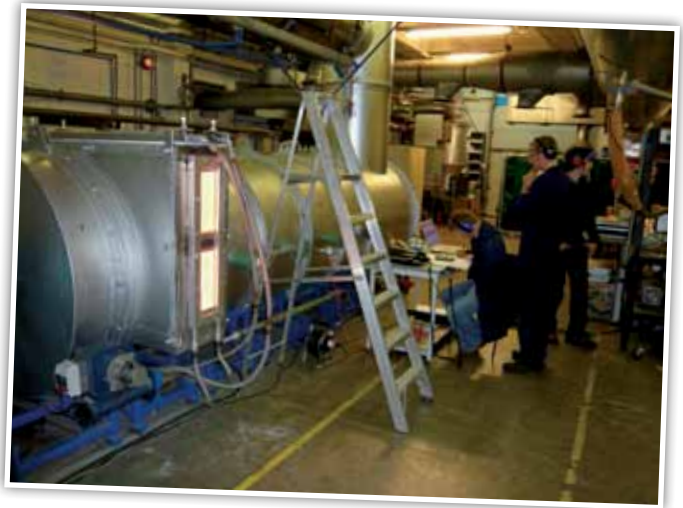
Laborelec and the University of Cardiff conducted atomization tests and established the preheating requirements for each type of biofuel.
