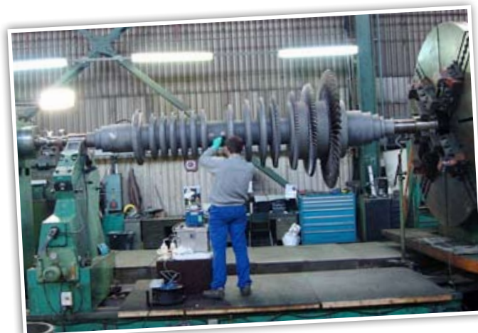
Steam turbine rotor during an inspection of one of the cracks.
