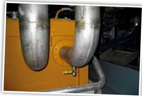
Good oil analysis requires proper oil sampling. Locations where the oil is very turbulent such as in a return pipe are excellent for collecting samples.
