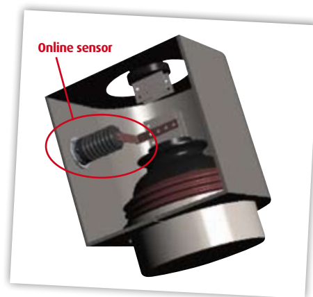
Laborelec simulates the specifics of the turbo-generator to determine the best location for online sensors.
