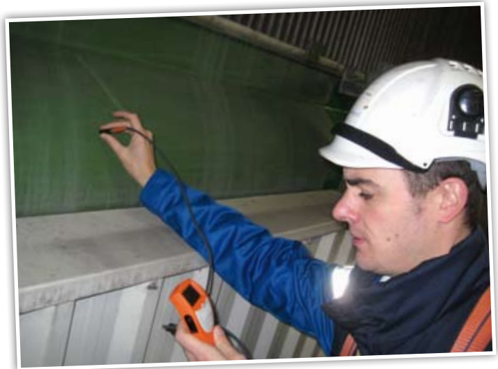
Measuring dry film thickness is one of the quality checks carried out by Laborelec.
