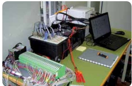
The Laborelec Steam Turbine Simulator tool.
