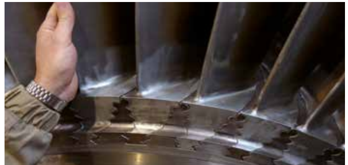
Our method makes it possible to carry out the inspection without dismantling of the rotor.
