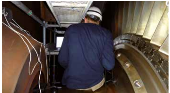
Our method makes it possible to carry out the inspection without dismantling of the rotor.
