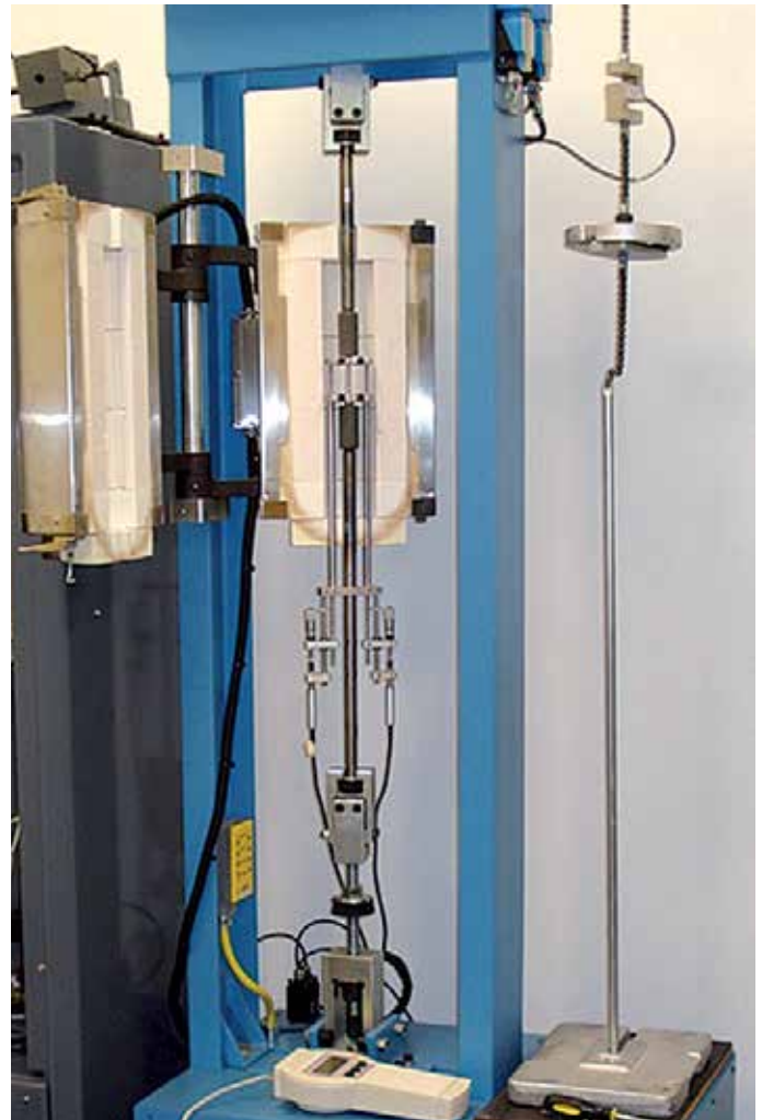
Laborelec's own creep testing facility for accelerated creep tests
