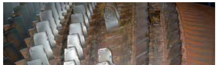
Compressor blade failure due to fatigue
