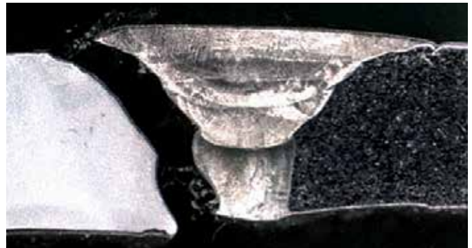
Dissimilar weld failure between T91 and 347H material
