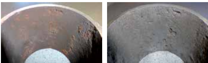
Evaporator tube sample before and after deposit removal test
